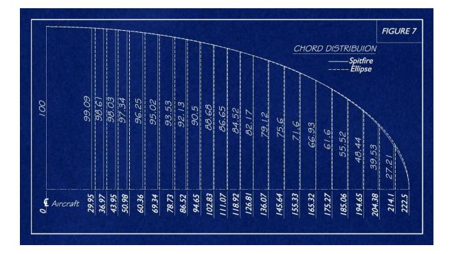
The chord distribution does not conform to an elliptic outline. How does one now retrace back to the original ellipse and figure out what exactly happened in terms of the quasi-elliptical or near
