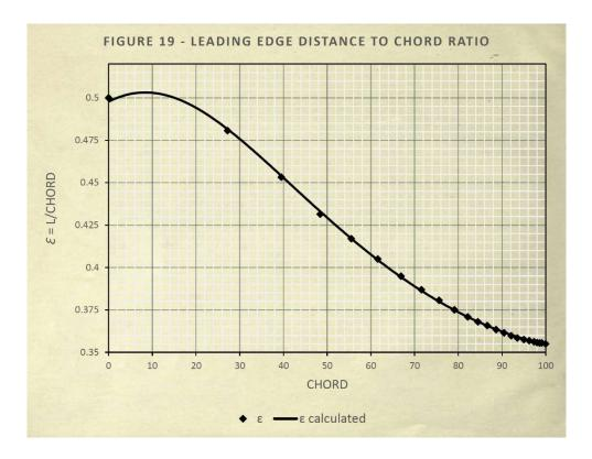
Figure 19 shows the Leading Edge 'L' distance to Chord ratio versus Chord as the Chord varies along the semi span. Offsets 'A' are from the front spar and are renamed 'L' as leading edge distance from wing axis ('A' + 11 inches) and the tabulated values are shown in Table 8.
