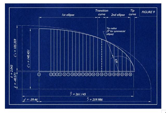
Station 16 chord is assumed to have been originally interpolated and therefore left unaltered. The result is shown in Table 5 and Figure 9.
