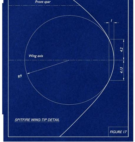
The chords are positioned about the wing axis is such a way that this ratio changes from 35.5% to 50% by a certain rule. For the Spitfire wing this can be plotted using leading edge offsets 'A' as per Supermarine drawing no. 337 08 SHT 8.
