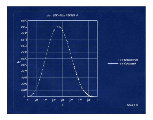
The leading edge points were first normalized (where root chord and span had a value of unity). A circular arc was then superimposed and the value of 1 was then subtracted from the radial distances of the leading edge points. This is shown in Figure 20. A probability curve called Beta Distribution (probability distribution) was iteratively fitted to these differences,  $\Delta r$  with respect to  $\theta$ . This is shown in Figure 21.
