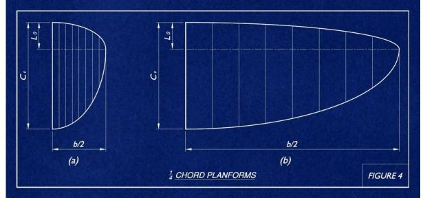
Consider an ellipse of similar eccentricity to the Spitfire wing with the ratio of b/2 to C at 4:1. The ratio of b/2 to C in Figure 4 (a) is 1:2. Multiplying the horizontal distances between the vertical chords by 8 will result in Figure 4 (b). This resulting shape also consists of two quarter ellipses and the chord distribution will again be elliptical.
