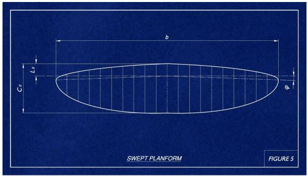
a curved or different sweep axis) has the same area as the planform in Figure 4 (b). This is analogue to the area of a parallelogram.
