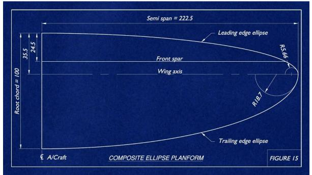
the wing aerodynamic centre and the 'D' wing leading edge together with the spar had to have sufficient chord-wise depth for adequate strength among other things.
