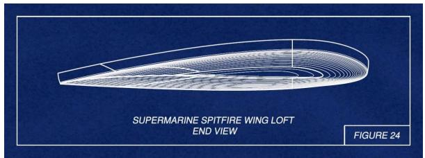
Figure 24 shows lofted airfoils looking along the dihedral plane (end view on Figure 18). Note the front and rear spar lines.
