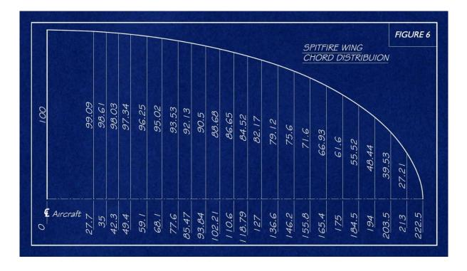
While the chords were kept the same, the semi-span column in Table 2 was calculated from Equation 1 as follows:
